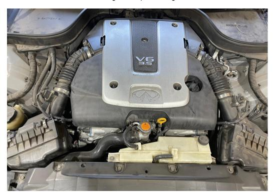
2. Using pliers, slide the clamp retaining the hose on the driver side valve cover off of its barb, do the same for the crossover hose on the front of the fitting.
