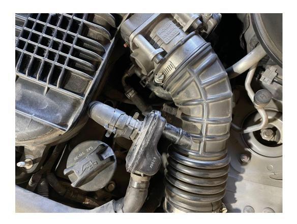
3. Remove the OEM plastic vacuum chamber from both intake tubes. (The couplers on the car we were installing them on were cracked so we went ahead and replaced both with the CZP silicone intakes)
